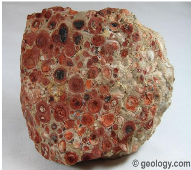
Fig: 1 Bauxite from little rock exhibiting a pistolic structure and characteristic red iron staining
