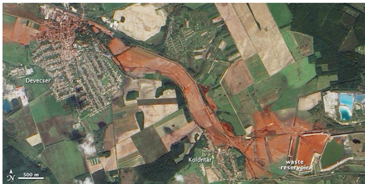
Figure 1. Red mud contaminated areas of Kolontár and Devecser villages in Central Transdanubia region of Hungary after the rupture of cassettes No 10 (waste reservoir) at waste red mud reservoir of MAL Co. Ltd. alumina plant in October 4 th , 2010 [8].
